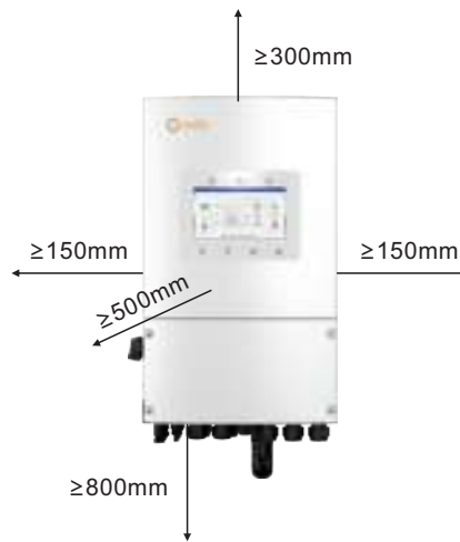
Figure 3.5 Inverter Mounting Clearances
