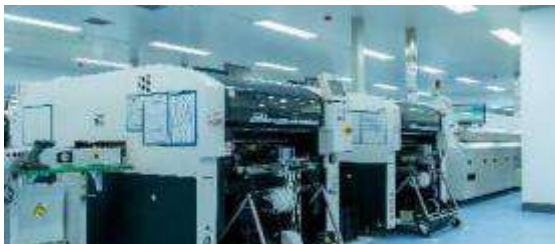
Surface Mounted Technology Machine
