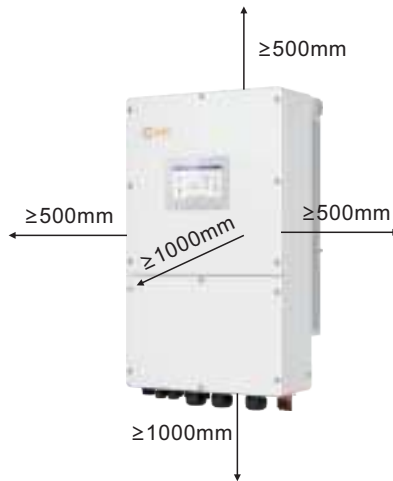
Figure 3.5 Inverter Mounting Clearances
