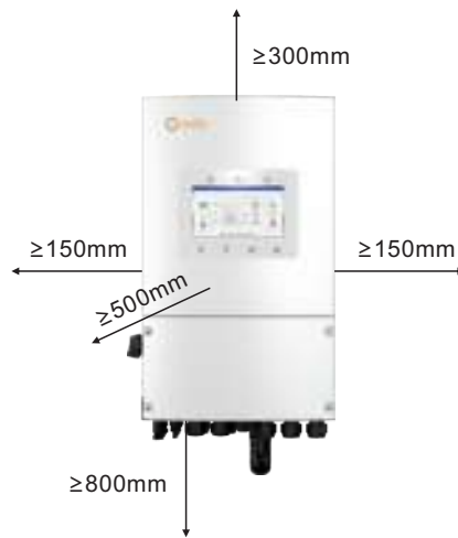
Figure 3.5 Inverter Mounting Clearances
